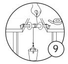
Holding on to the loose end of string so that your spool doesn't unwind, tape the ends of the pencil to the surface where you wish to mount your pulley.
